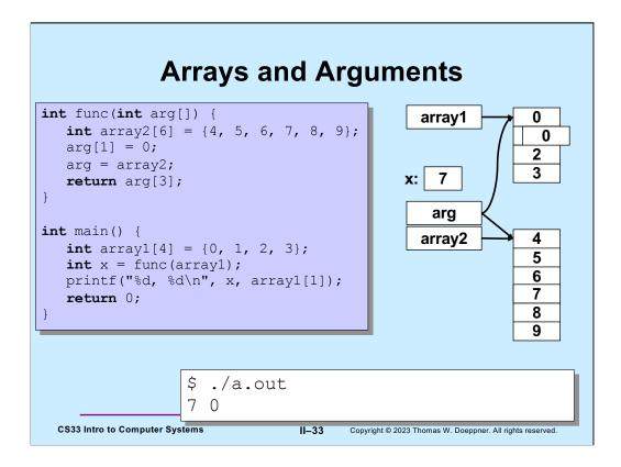
In this example, we've declared **array1** and **array2** in **main** and **func**. Both declarations allocate storage for arrays of **int**s. Both **array1** and **array2** refer (by pointing to the first elements) to the storage allocated for the arrays. What memory locations they refer to can't be changed (though the contents of these locations can be changed).
