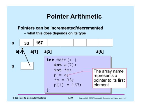
A pointer to the first element of an array can be used as if it were the array itself. Thus, in this example, there's little difference between how one uses "p" and "a".
