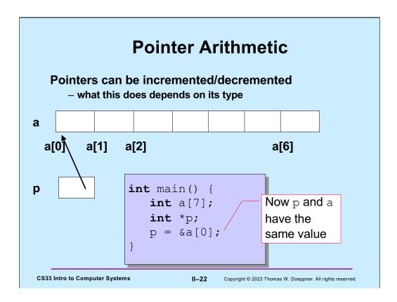
Note that setting  $\mathbf{p}$  equal to the address of the first element of the array a is equivalent to setting  $\mathbf{p}$  to the value of  $\mathbf{a}$ .
