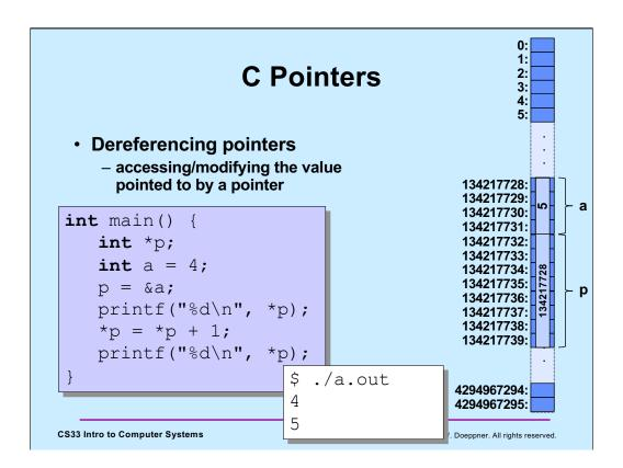
Keep in mind that though we are changing p's value (by assigning to it the address of a), we are not changing the memory address associated with p – it remains 134217732 (and its size remains 8).
