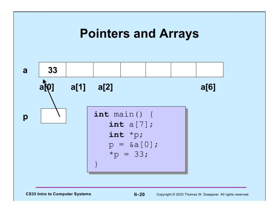
The pointer p points to the first element of the array a. Thus a[0] and \*p have identical values.
