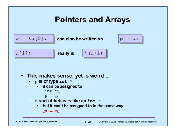
The name of a local array represents a pointer to its first element. But we treat this pointer as a constant – it can't be modified (if we did so, what would we do with the storage that it previously pointed to?)
