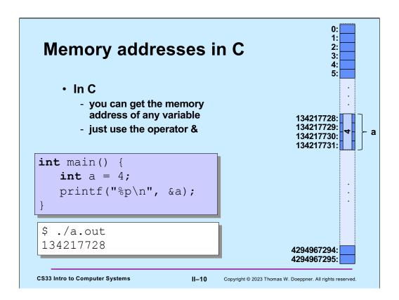
The "%p" format code in printf means to interpret the item being printed as being a pointer.
