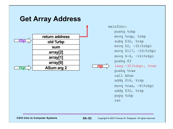
In preparation for pushing the first argument to **ASum** onto the stack, the address of the array is put into %rax.
