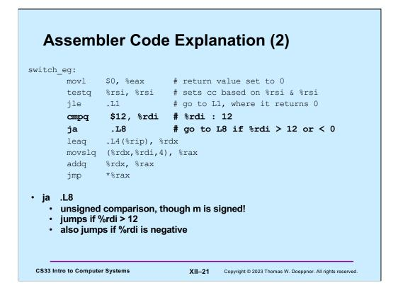
The next two instructions simply check to make sure that %rdi (the first argument, m) is less than or equal to 12. If not, control goes to .L8, which sets the return value to 0 and returns. Of course, the return value (in  $\frac{\pi x}{\theta eax}$ ) is already zero, so setting it to zero again is unnecessary.
