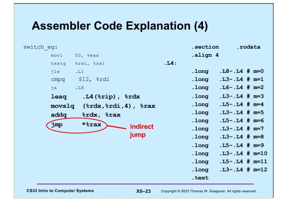
The highlighted code makes use of an indirect jump instruction, indicated by having an asterisk before its register operand. The register contains an address, and the jump is made to the code at that address. Note that jump instructions that are not indirect have constants as their operands. We'll see later on that, because of this, indirect jumps are often much slower than non-indirect jumps.
