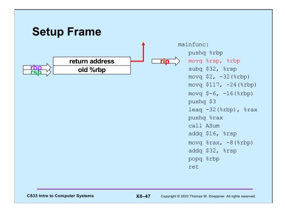
The first thing done by **mainfunc** is to save the caller's %rbp by pushing it onto the stack.
