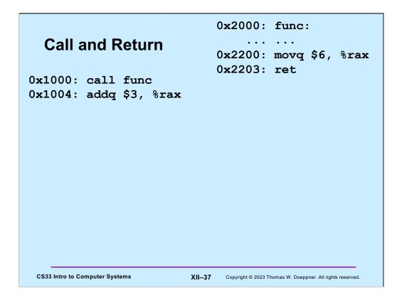
When a function is called (using the **call** instruction), the (8-byte) address of the instruction just after the **call** (the "return address") is pushed onto the stack. Then when the called function returns (via the **ret** instruction), the 8-byte address at the end of the stack (pointed to by %rsp) is copied into the instruction pointer (%rip), thus causing control to resume at the instruction following the original call.
