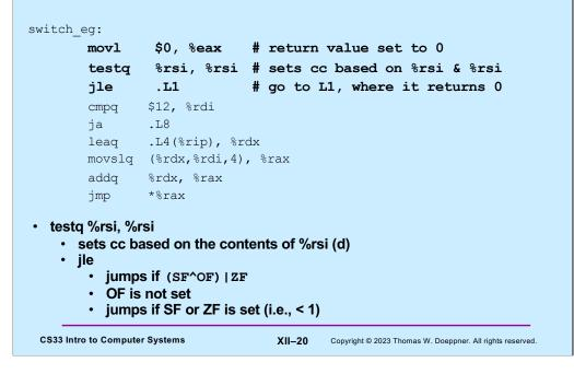
The first three instructions cause control to go to .L1 if the second argument (d) is less than 1. At .L1 is code that simply returns (with a return value of 0).
