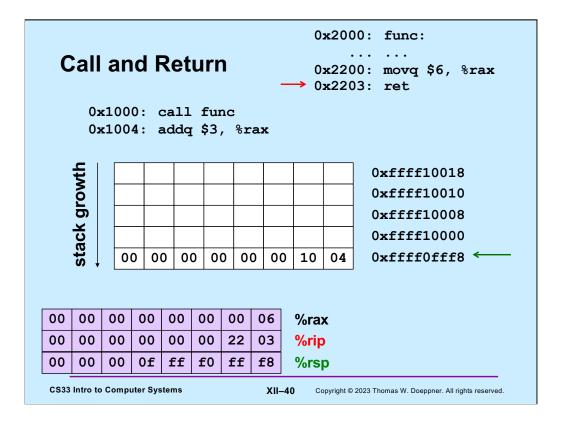
Our function **func** puts its return value (6) into %rax, then executes the **ret** instruction. At this point, the address of the instruction following the **call** is at the end of the stack.
