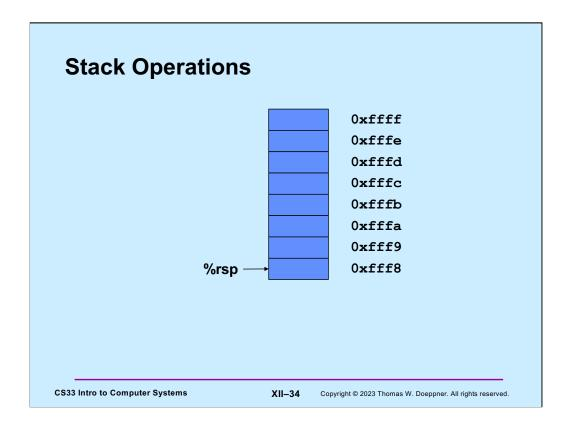
The stack-pointer register (%rsp) points to the last byte of the stack. Thus, with littleendian addressing, it points to the least-significant byte of the data item at the end of the stack. Thus, %rsp in the slide points to what's perhaps an 8-byte item at the end of the stack.
