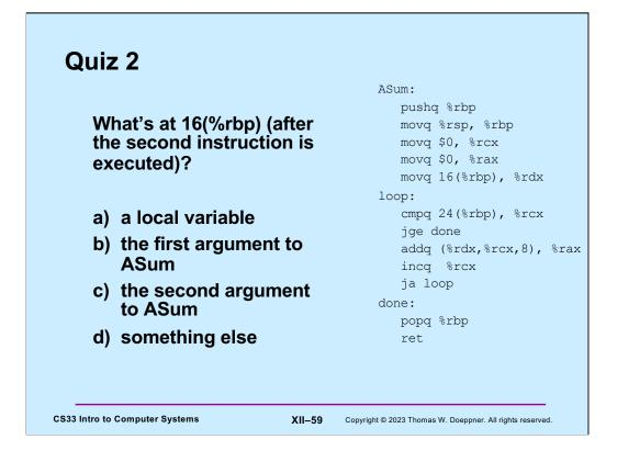
Recall that when the function was entered, %rsp pointed to the return address (on the stack). It now points to something that's 8 bytes below that. Also recall that arguments to a function are pushed onto the stack in reverse order.
