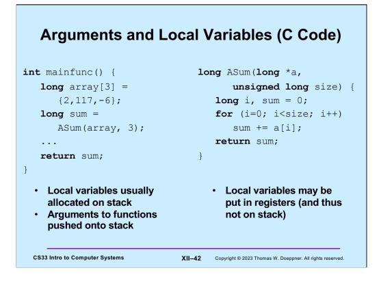
We explore these two functions in the next set of slides, looking at how arguments and local variables are stored on the stack. Note that the approach of storing arguments on the stack is used on the IA32 architecture, and on the x86-64 architecture when the – O0 optimization flag (meaning no optimization) is given to gcc.
