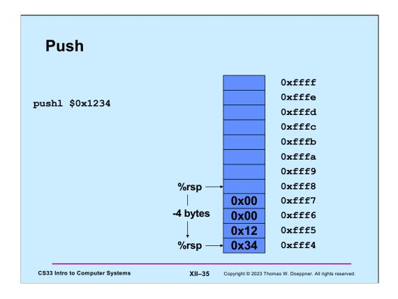
Here we execute **push1** to push a 4-byte item onto the end of the stack. First %rsp is decremented by 4 bytes, then the item is copied into the 4-byte location now pointed to by %rsp.
