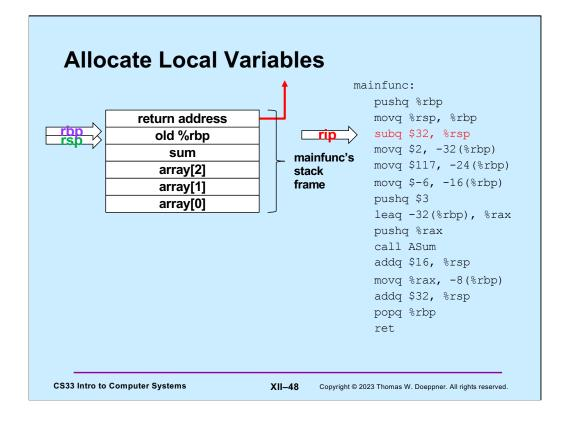
Next, space for **mainfunc**'s local variables is allocated on the stack by decrementing %rsp by their total size (32 bytes). At this point we have **mainfunc**'s stack frame in place.
