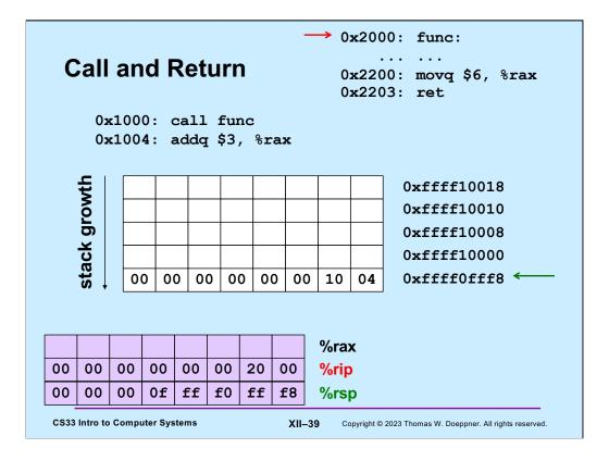
When the **call** instruction is executed, the address of the instruction after the **call** is pushed onto the stack. Thus %rsp is decremented by eight and 0x1004 is copied to the 8-byte location that is now at the end of the stack. The instruction pointer, %rip, now points to the first instruction of **func**.
