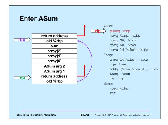
As on entry to **mainfunc**, %rbp is saved by pushing it onto the stack.
