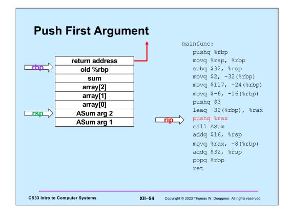
And finally, the address of the array is pushed onto the stack as **ASum**'s first argument.
