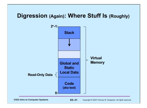
Here we revisit the slide we saw a few weeks ago, this time drawing it with high addresses at the top and low addresses at the bottom. The point is that a large amount of virtual memory is reserved for the stack. In most cases there's plenty of room for the stack and we don't have to worry about exceeding its bounds. However, if we do exceed its bounds (by accessing memory outside of what's been allocated), the program will get a seg fault.
