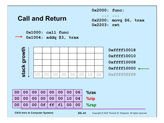
The address at the end of the stack (0x1004) is popped off the stack and into %rip. Thus execution resumes at the instruction following the **call** and %rsp is incremented by 8, The function's return value is in %rax, for access by its caller.
