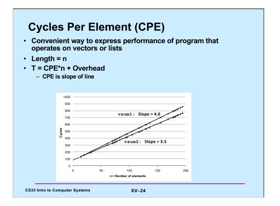
A **cycle** is a measure of processor time, often referred to as a **clock cycle**. Processors are driven by a clock, running at a certain frequency, say 10 GHz ( $10^{*}2^{30}$  cycles per second). In this case, the length of a cycle is the period of the clock (the reciprocal of its frequency -  $.1^{*}2^{-30}$  seconds).
