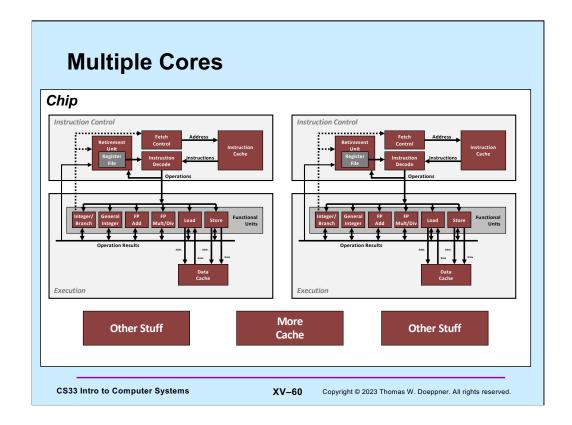
Going a step further, one can pack multiple complete processors onto one chip. Each processor is known as a core and can execute instructions independently of the other cores (each has its private set of functional units). In addition to each core having its own instruction and data cache, there are caches shared with the other cores on the chip. We discuss this in more detail in a subsequent lecture.
