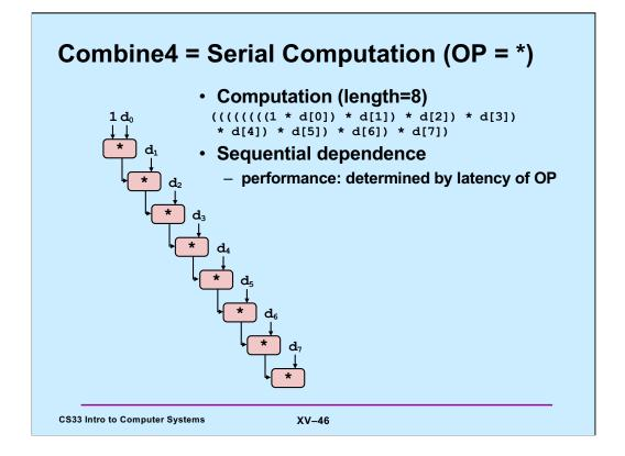
Since the multiplies form the critical path, here we focus only on them. In what's shown here, only one multiply can be done at a time, since the result of the one multiply is needed for the next.
