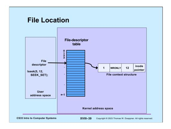
One can set the file location by using the lseek system call. Setting it will affect where the next read or write takes place. If the third argument is SEEK\_SET, the offset given in the second argument is treated as an offset from the beginning of the file. If it's SEEK\_CUR, it's treated as an offset from the current position in the file. If it's SEEK\_END, it's treated as an offset from the end of the file.
