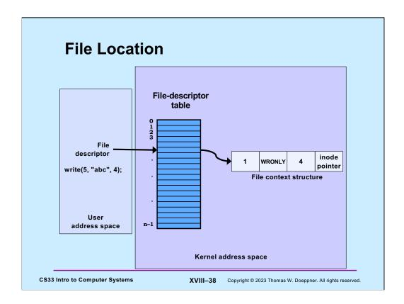
After reading or writing n bytes to a file, its file-location value is incremented by n. Thus, by default, I/O to files is sequential.
