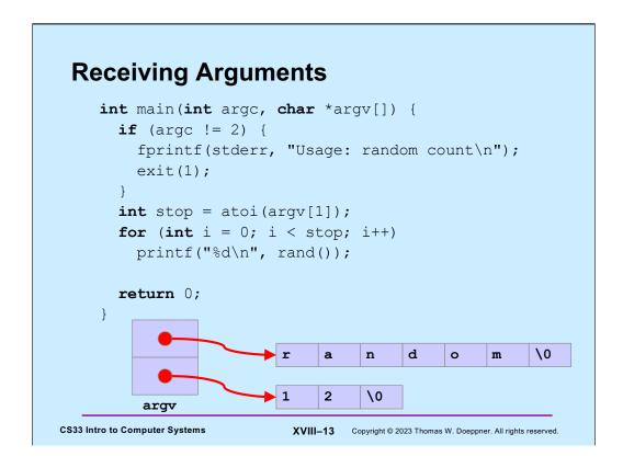
Note that argv[0] is the name by which the program is invoked. argv[1] is the first "real" argument. In this program, argv[2] will contain the NULL pointer (0). arrgc is two, indicating two arguments (argv[0] and argv[1]).
