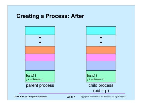
By executing **fork** the parent process creates an almost exact clone of itself that we call the child process. This new process executes the same text as its parent, but contains a copy of the data and a copy of the stack. This copying of the parent to create the child can be very time-consuming if done naively. Some tricks are employed to make it much less so.
