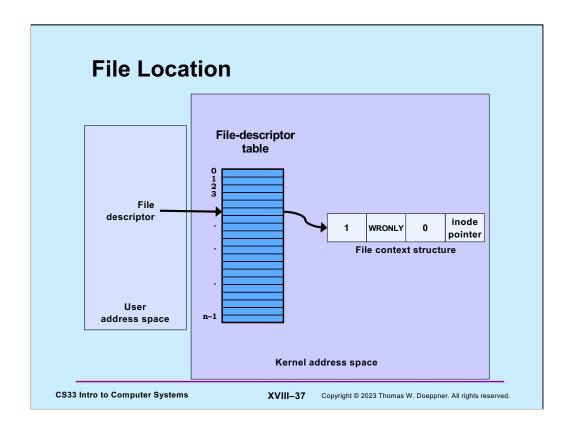
The file-location field in the context structure indicates the offset into the file at which the next read or write operation will take place. It's normally set to 0 by OS when the file is opened (one can also have it set to the offset of the end of the file by setting the O\_APPEND flag in open).
