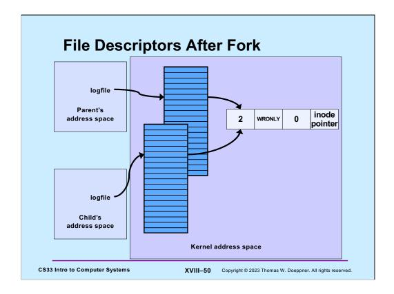
Note that after a **fork**, the reference counts in the file context structures are incremented to account for the new references by the child process.
