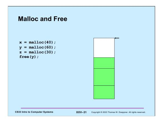
The arrow points to the current program break, indicating the end of the dynamic region. We want to use **malloc** and **free** to manage the memory in the current dynamic region.
