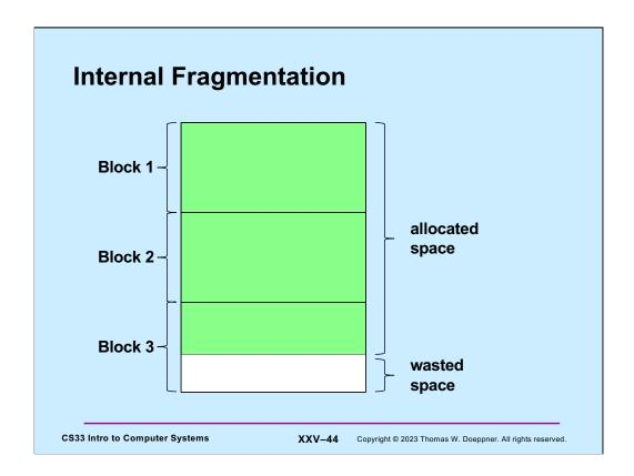
While this isn't important for this course, internal fragmentation occurs when memory is allocated in fixed-size blocks, say 4k bytes each. If we allocate space for a data structure whose size is not a multiple of the block size, the wasted space is said to be due to **internal fragmentation**.
