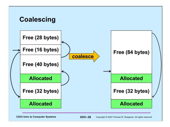
The solution is known as **coalescing**: when freeing a block, we look at adjacent blocks. if either or both adjacent blocks are free, we merge the newly freed block with its non-allocated neighbors to form a single free block whose size is the sum of the sizes of the blocks being coalesced.
