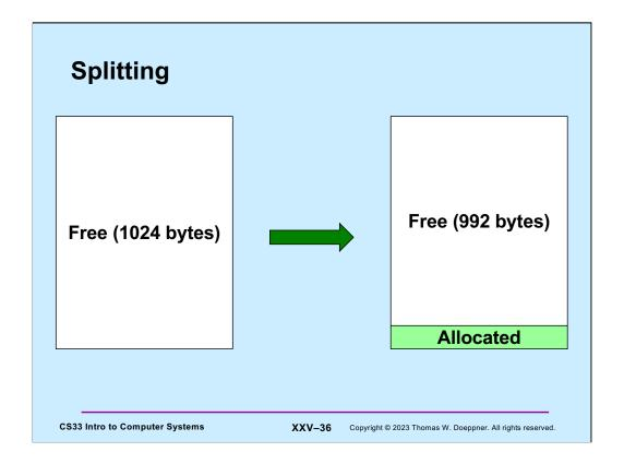
It makes no sense for malloc to return a block that's much larger than needed. Instead, it should split the block into two pieces: one piece is returned to the caller and is at least as large as was requested. The other piece is put back on the free list with an adjusted size.
