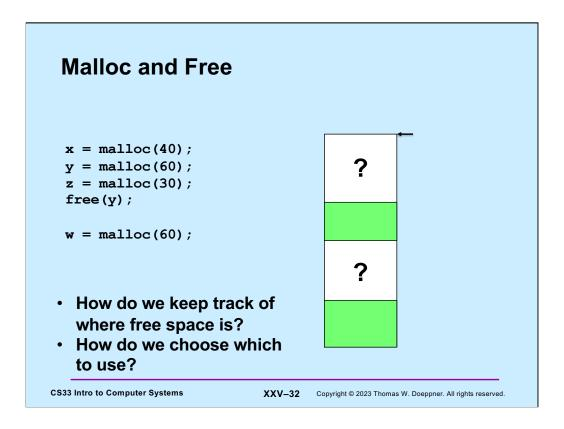
Somehow we need to keep track of where the free space is, so we can use it to handle allocation requests. The green areas of memory are allocated, the white areas are unallocated.
