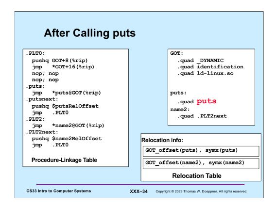
Finally, ld-linux.so writes the actual address of the **puts** procedure into the **puts** entry of the global-offset table, and, after unwinding the stack a bit, passes control to **puts**. On subsequent calls by the module to puts, since the global-offset table now contains **puts**'s address, control goes to it more directly, without an invocation of ld-linux.so.
