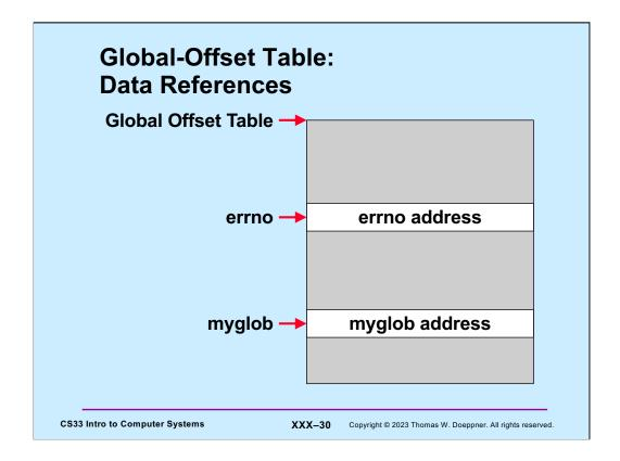
To establish position-independent references to global variables, the compiler produces, for each module, a **global-offset table**. Modules refer to global variables indirectly by looking up their addresses in the table, using PC-relative addressing. The item needed is at some fixed offset from the beginning of the table. When the module is loaded into memory, ld-linux.so is responsible for putting into it the actual addresses of all the needed global variables.
