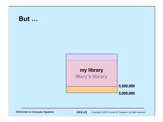
Pre-relocation doesn't work if we have two libraries pre-assigned such that they overlap. If so, at least one of the two will have to be moved, necessitating relocation.
