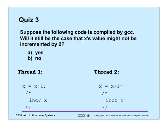
In this example, gcc generates an instruction that directly increments the memory location holding  $\mathbf{x}$ .
