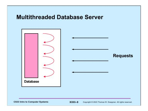
We now rearchitect our server to be multithreaded, assigning a separate thread to each request. The code is as simple as in the sequential approach and as fair as in the multiplexed approach. Some synchronization of access to the database is required, a topic we will discuss soon.
